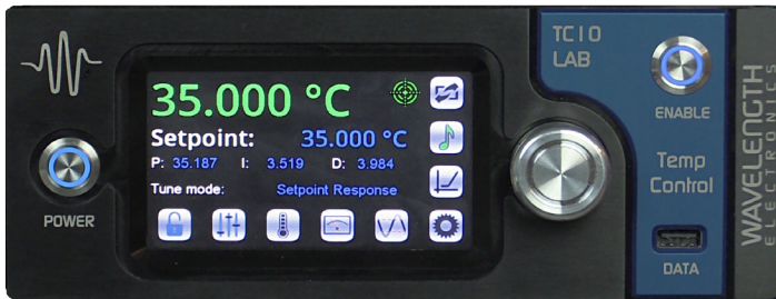
Figure 18. PID Coefficients automatically recalculated for setpoint change
