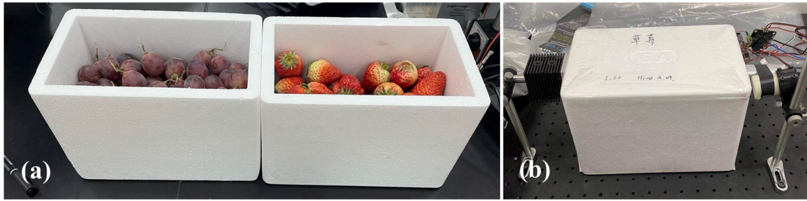
Fig. 2. Photographs of the experimental sample and set-up: (a) fruit boxes before being sealed; (b) sealed fruit box under study, with the PMT placed on one side of the box and the laser directed from the other side.
